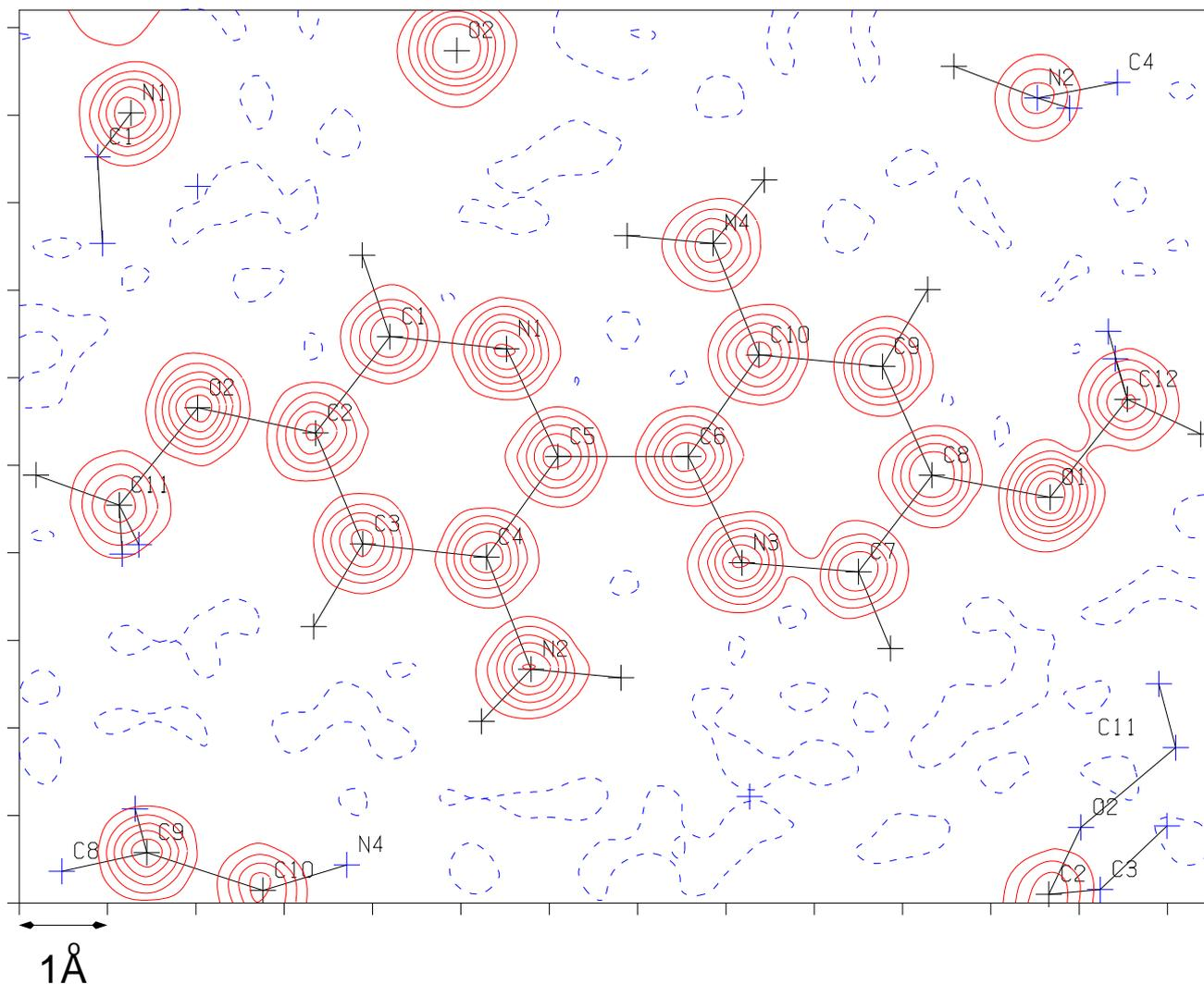
Contour plot of the electron density in the least-squares plane through 5,5'-dimethoxy-3,3'-diamine-2,2'-bipyridine. Lines are drawn at intervals of 2.0 e Å<sup>-3</sup>; the dashed line represent the level of 0.0 e Å<sup>-3</sup>. A + indicates the position of an atom within 1.0 Å of the plane.
