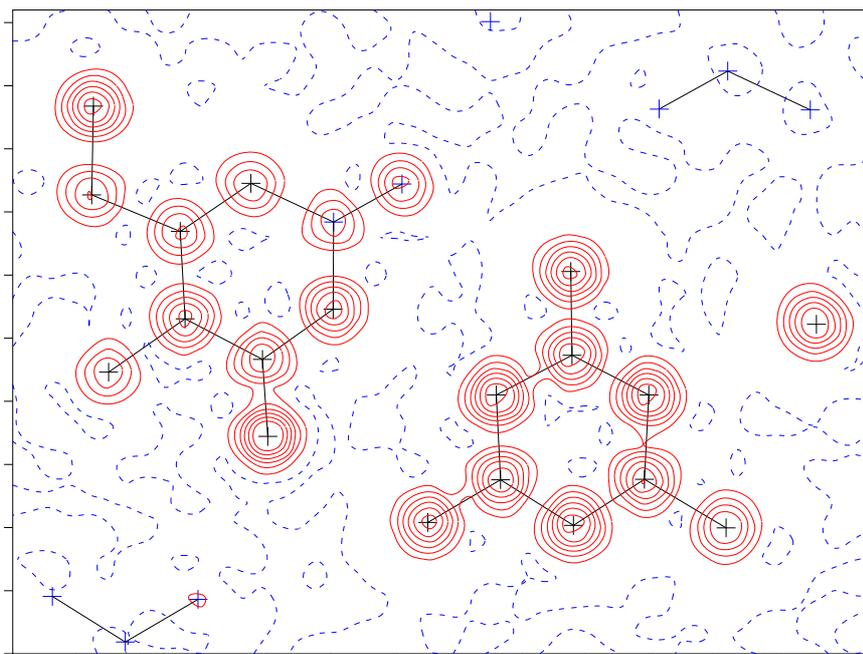
$\rho(x, y, z)$  for a model without hydrogen atoms (contour interval  $2 \text{ e } \text{\AA}^{-3}$ )
