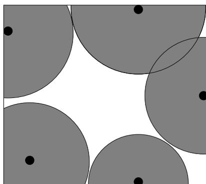
2. Add the radius of the smallest possible solvent (water,  $r = 1.2 \text{ \AA}$ ) to the excluded volume of step 1. The remaining volume (white) is accessible for the nucleus of the solvent.
