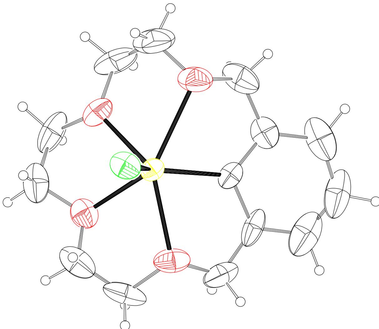
drawn at 30% probability level, meaning that the chance of finding the atomic nucleus within the plotted ellipsoid is 30%.
