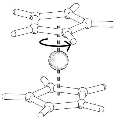
With this technique the cyclopentadiene rotation barrier around the (local) 5-fold axis in ferrocene was found to be in the range 7.6(2)–9(2) kJ mol<sup>-1</sup> at 101K; in good agreement with results obtained by other techniques.
