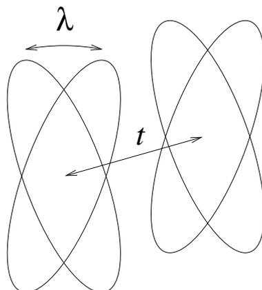
Librational and translational parameters are fitted to the observed  $U_{ij}^{\text{obs}}$  with a least-squares procedure. With the obtained translation ( $T$ ), libration ( $L$ ) and correlation ( $S$ ) tensors, the TLS model values  $U_{ij}^{\text{calc}}$  can be calculated. The validity of the TLS model can be assessed by comparing  $U_{ij}^{\text{obs}}$  and  $U_{ij}^{\text{calc}}$  via R-values.
