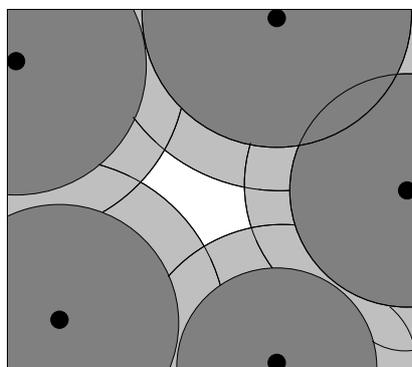
3. Add the radius of the smallest possible solvent to the remaining volume of step 2. The solvent accessible volume is indicated in white.
