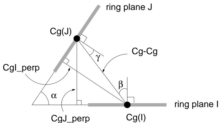
where  $Cg$  is the geometrical centre of the ring. The geometry is analyzed when  $Cg-Cg < 6.0 \text{ \AA}$  and  $\beta < 60^\circ$ .
