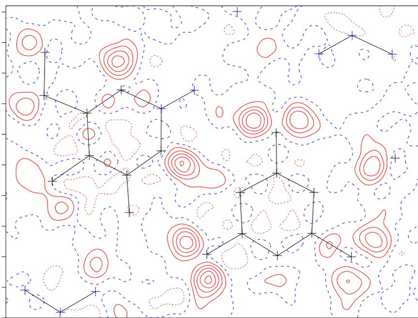
$\Delta\rho(x, y, z)$  for the same model (contour interval  $0.15 \text{ e } \text{\AA}^{-3}$ )
