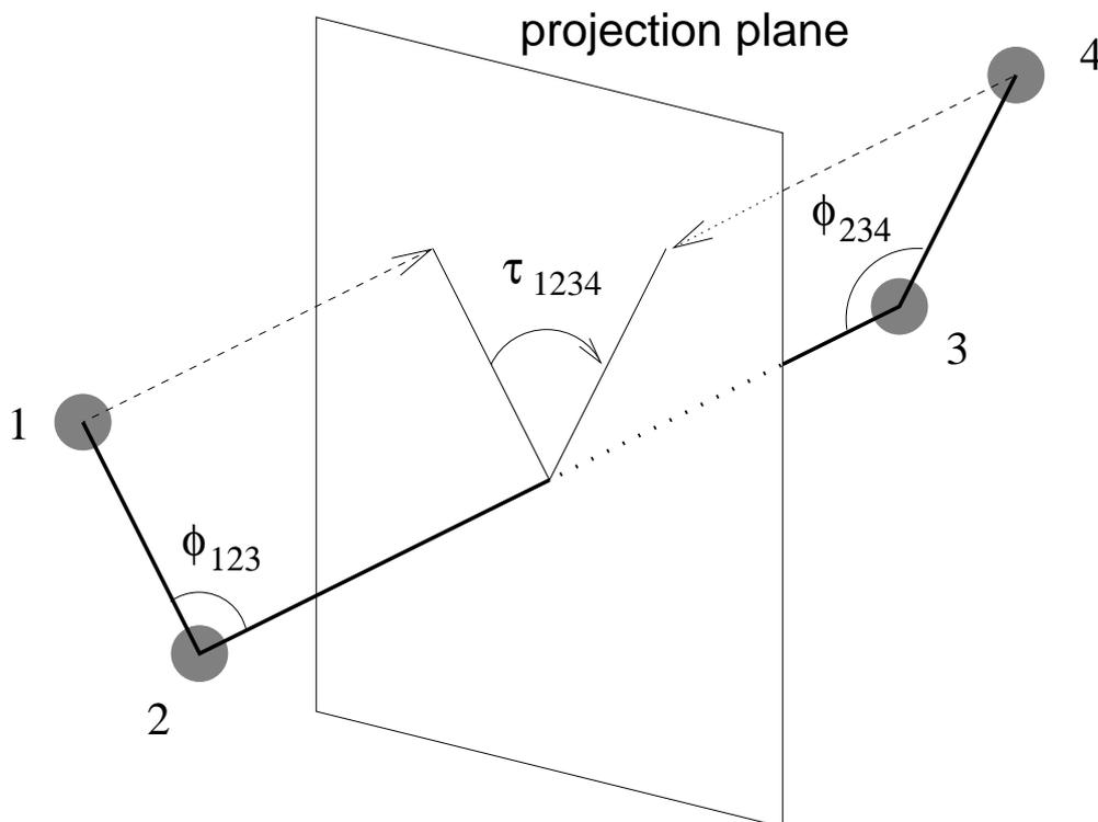
The torsion angle is calculated as the angle between the normal vectors to the plane through atoms 1, 2 and 3 and the plane through atoms 2, 3 and 4:
