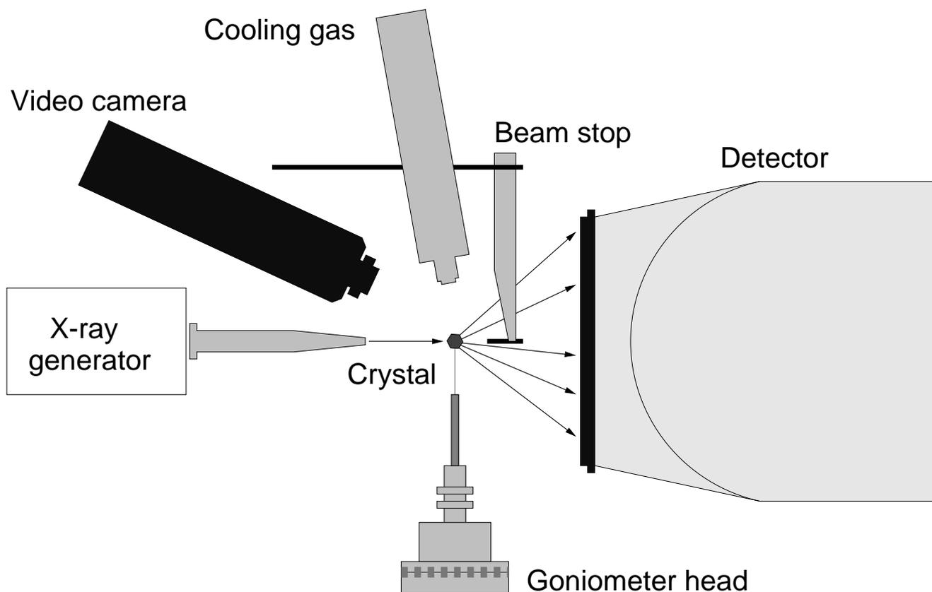
X-ray generator: molybdenum rotating anode (60kV, 50 mA), fine focus primary beam ( $\varnothing$  0.3 mm), wavelength  $\lambda_{\text{MoK}\alpha} = 0.71073 \text{ \AA}$ .
