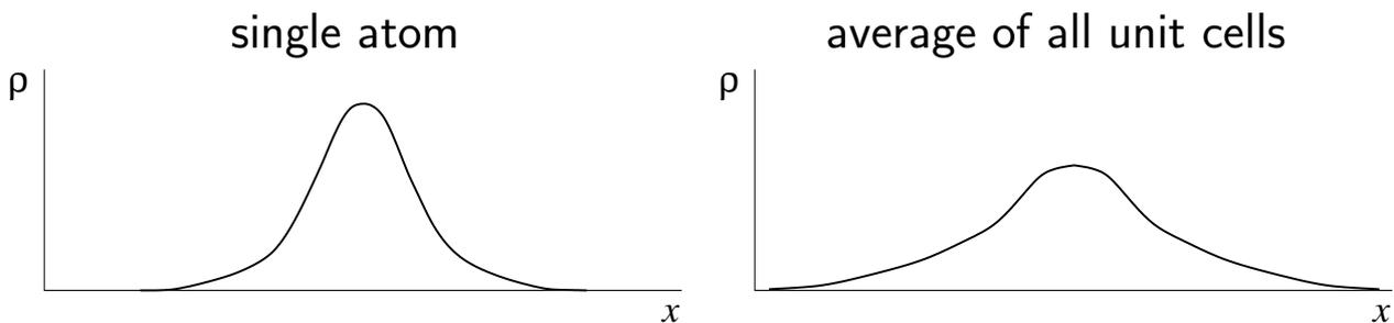
A displacement correction (formerly called temperature correction) has to be added to the scattering factor. Like  $f^0$ , the correction is a function of  $\sin \theta / \lambda$ :
