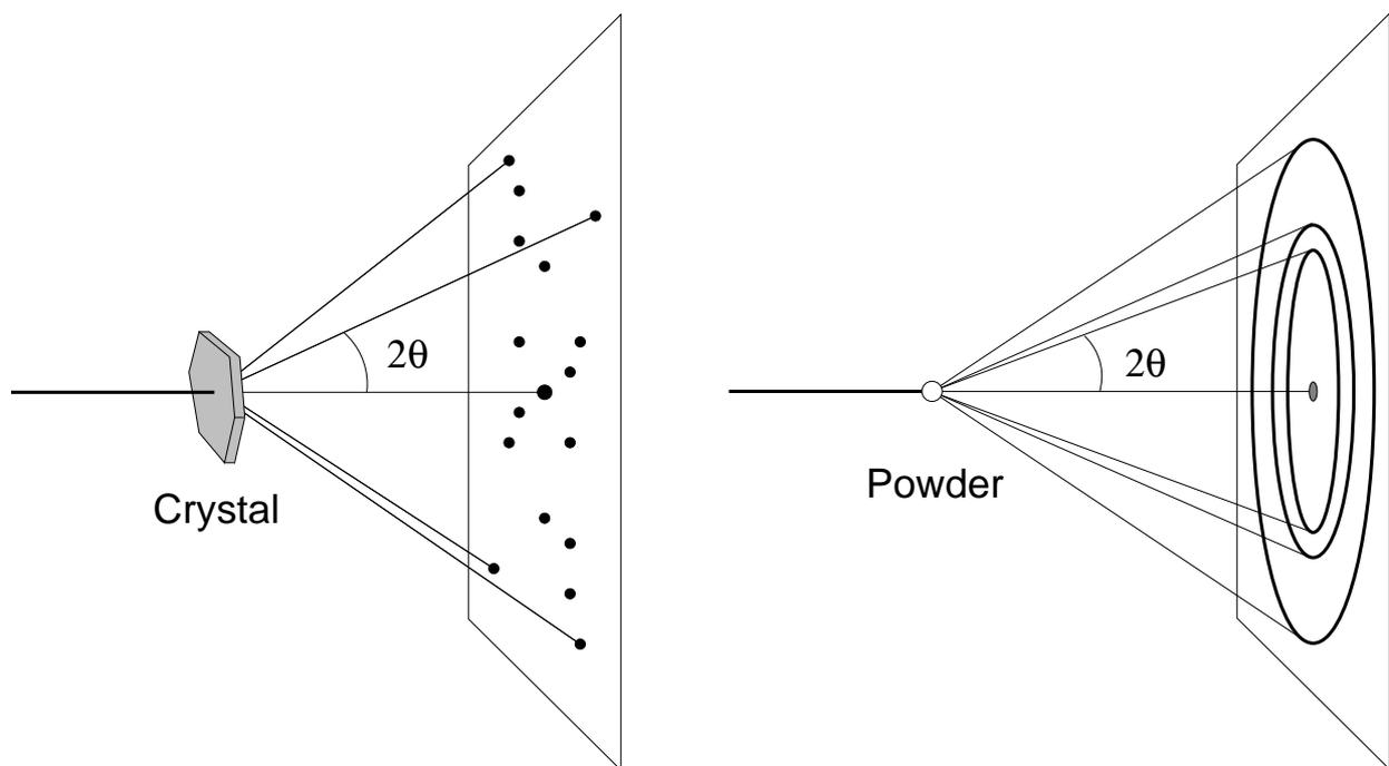
The diffraction pattern of a single crystal will change when the sample is rotated. The diffraction pattern of a powder will keep the same appearance when the sample is rotated, although other powder grains will contribute to the pattern.
