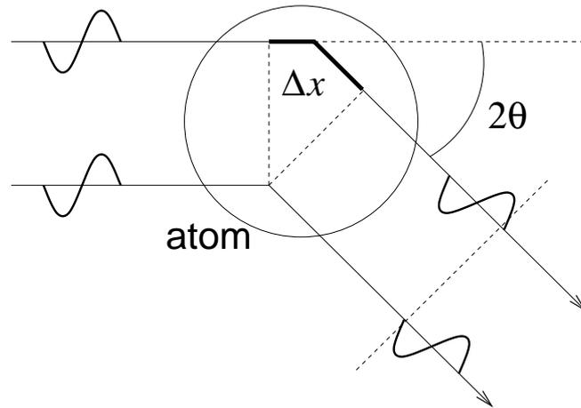
The amount of radiation scattered in each direction is described with the scattering factor  $f$ , also called form factor.
