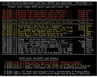
Figure 6 PLATON/checkCIF report: (a) structural data summary and (b) ALERT listing.
