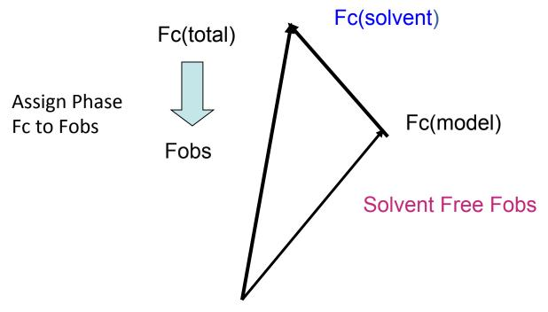
Black: Split Fc(total) into a discrete atom and solvent contribution Red: For SHELX refinement, temporarily substract the recovered solvent contribution from Fobs. (To be reinstated after convergence)
