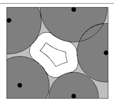
Black areas indicate discrete model atom with van der Waals radii assigned. The white area is the solvent accessible volume
